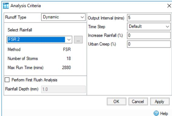
4. The Rainfall used in the **Analysis Criteria** can be altered by selecting the ... button to edit. This opens up the **Rainfall Manager**, within here a variety of rainfall types can be created, amended, or imported into the software to be used for analysis.
