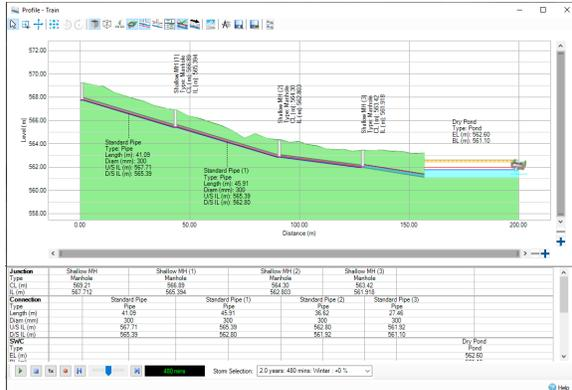
19. We can also run simulations for the 1:30 year storms, which can be done by changing the rainfall in **Analysis Criteria**. Change the rainfall to **FSR 30** and rerun the analysis.
