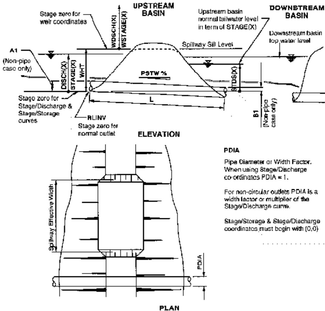
Puls' level pool routing technique is used to route the inflow hydrograph through the nominated storages. A stage storage relationship is defined for each of the storages. The outlet structures that may be handled include:
