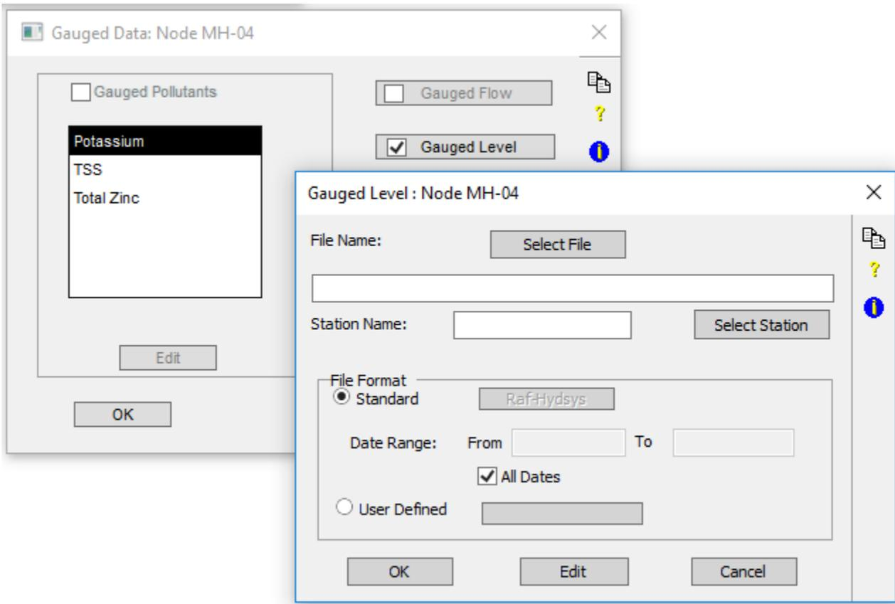
Gauge Pollutant graphing is available in the Runoff and Sanitary modes. Gauged Pollutants must be checked in the [Job Control](#) settings to enable tagging pollutant data to a node or link.
