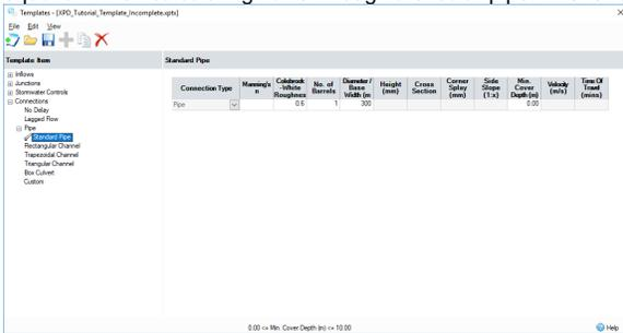
5. This process can be repeated to provide templates for any type of Inflow, Junction, Stormwater Control or Connection. Once you have created a Template, you can save the Template (\*.xptx) file for use in other designs. Further, you can Open or Import another Template file for use in your Design. Open will replace any pre-existing Template data, whereas importing a Template file will provide you with a list of Templates to Import to your Template list and merge the items available.
