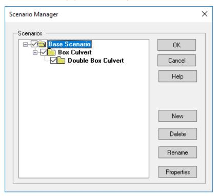
c. With the Box Culvert scenario highlighted, click New to add an additional scenario called Double Box Culvert.
